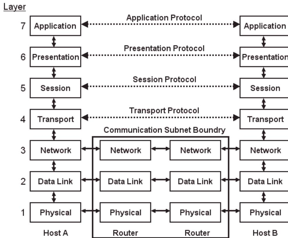
Figure 4: The ISO-OSI Reference Architecture
