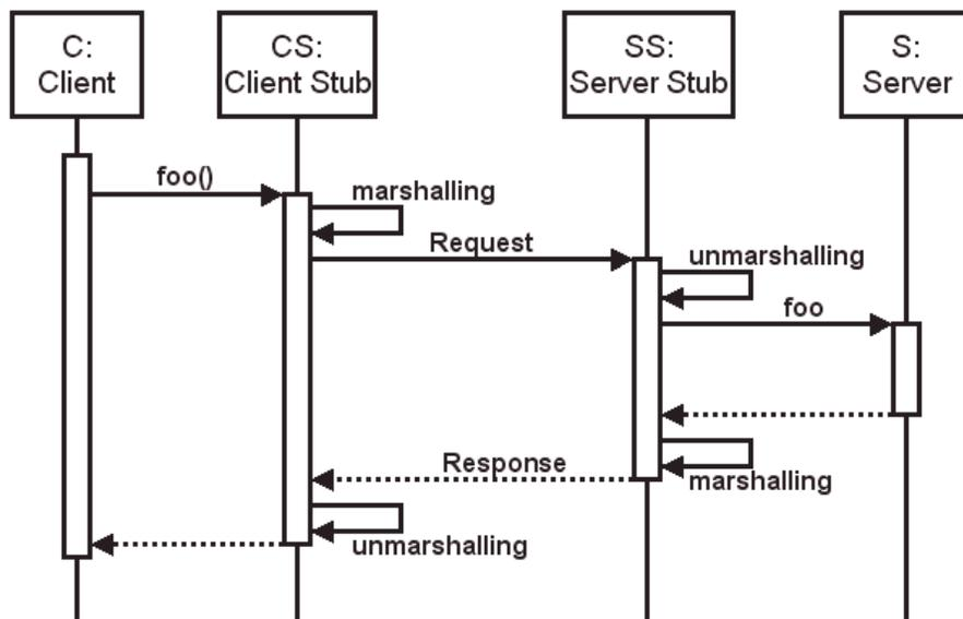
**Figure 8: Sequence Diagram Of A Remote Method Call**
