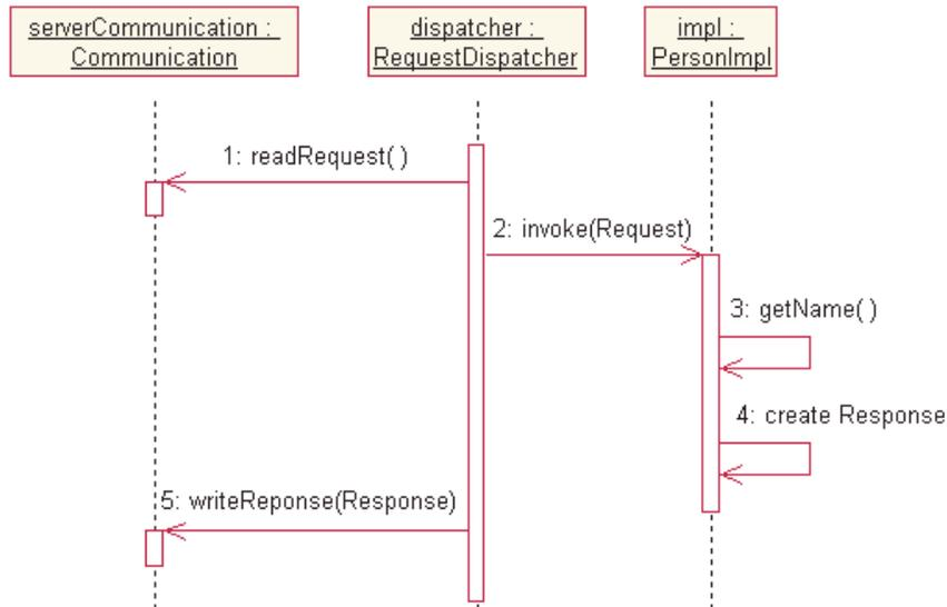
**Figure 13: Sample Dynamic Model Of A Remote Method Call (Server Side)**
