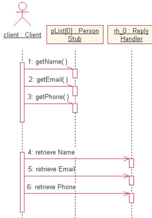
**Figure 41: Asynchronous Method Calls**
