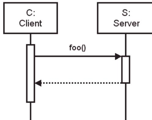
**Figure 2: Sequence Diagram Of A Local Method Call**
