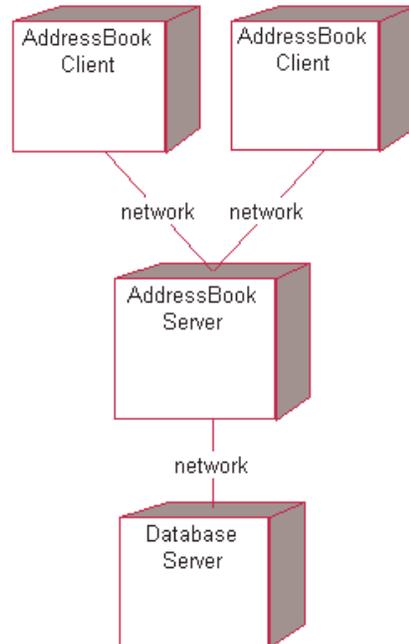
**Figure 47: Address Book Sample Deployment Diagram**
