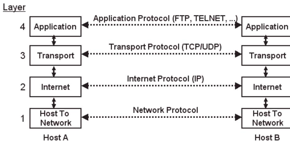
**Figure 5: The TCP/IP Reference Architecture**
