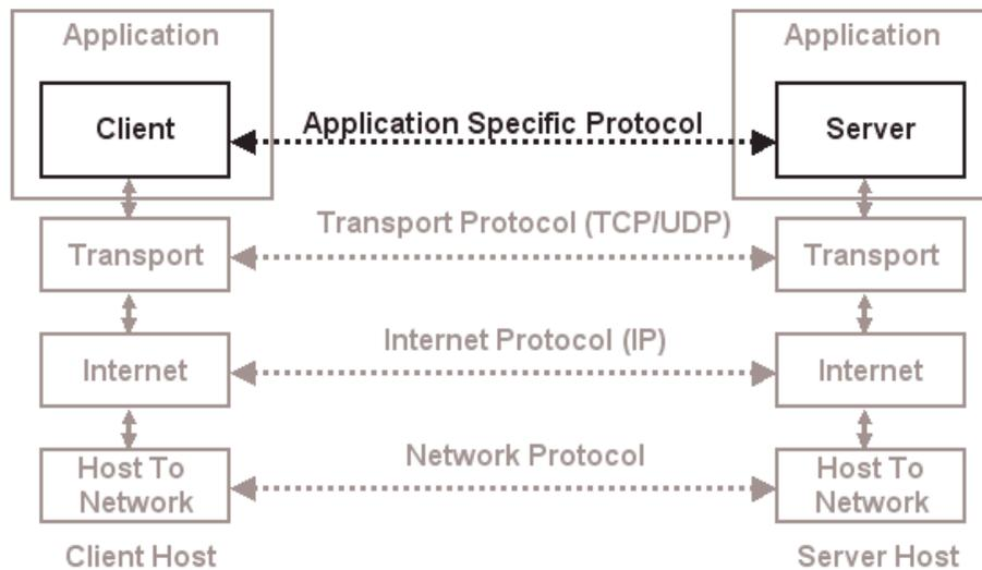
**Figure 6: TCP/IP Client/Server Communication**
