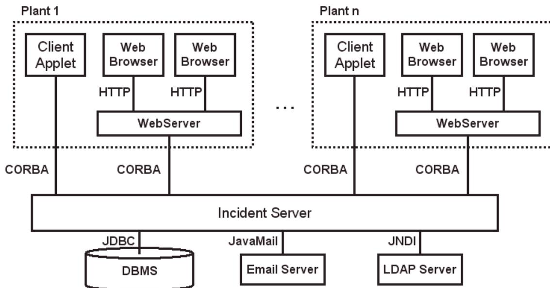
Figure 88: AQUA System Deployment
