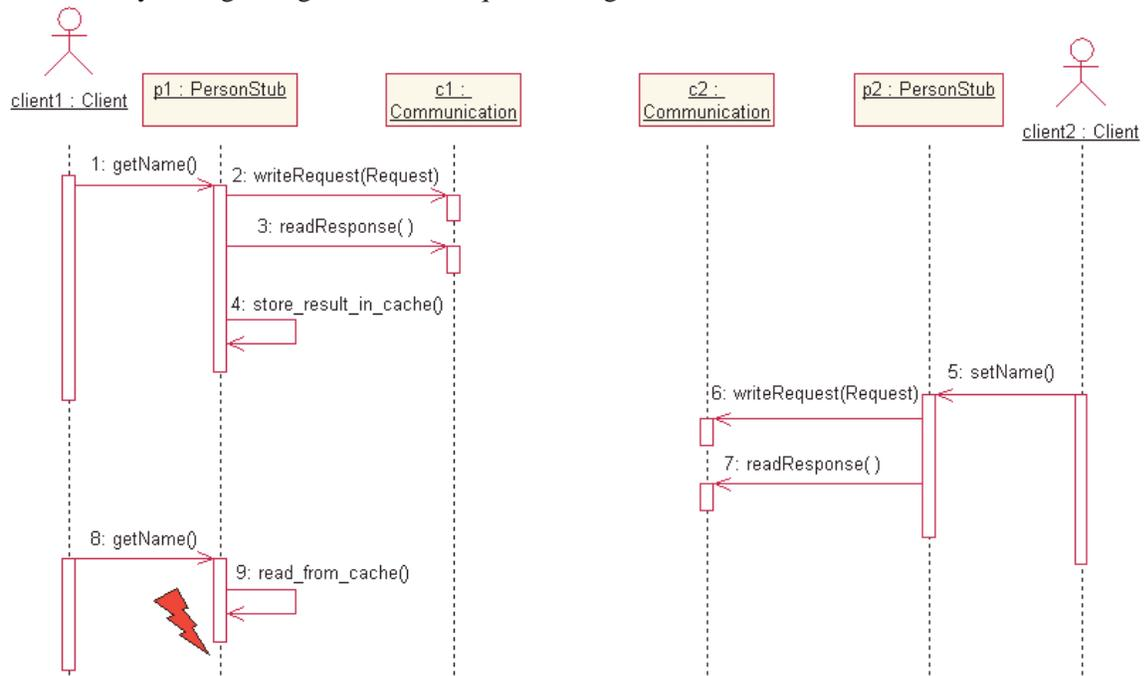
**Figure 50: Sequence Diagram Of System Inconsistency**
