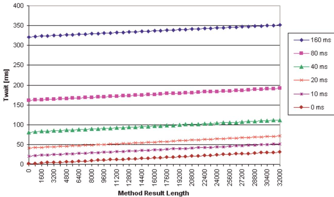
Figure 17: Twait For Different Network Delays
