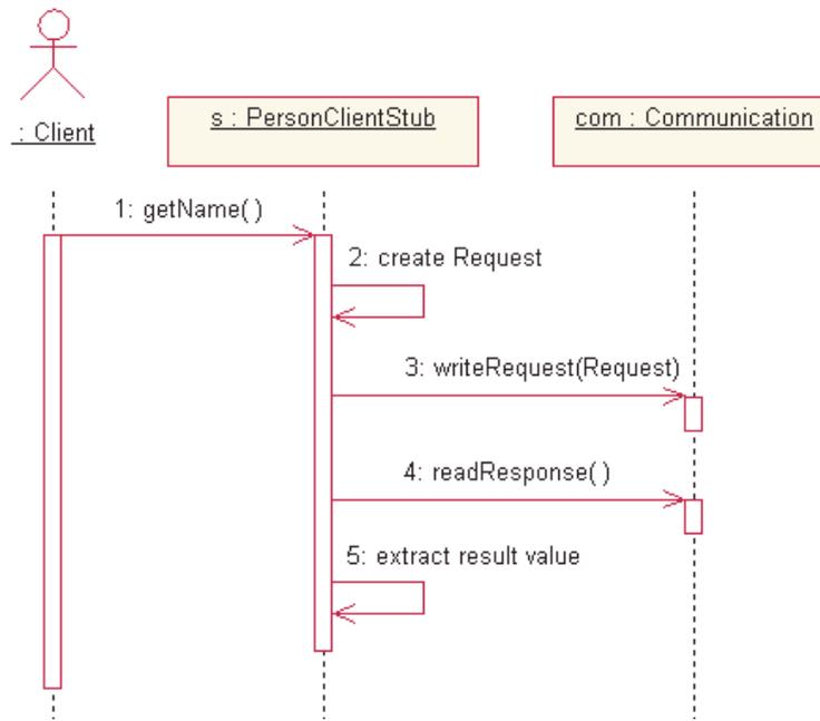
**Figure 12: Sample Dynamic Model Of A Remote Method Call (Client Side)**
